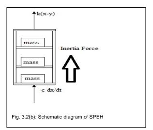
The analysis of forced vibrations due to excitation of support can be done considering absolute amplitude & relative amplitude of mass with respect to the support or base. In our case the nomenclature of various parameters is as follows:
