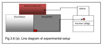
At a excitation frequency of 37 Hz the shaker is operated by amplifying the current to give different amplitudes to the shaker. Oscilloscope is used for measuring the output voltage of SPEH; it indicates the voltage on vertical axis and time in seconds on horizontal axis. Authors considered the time of hitting mass and measured the frequency. At the time of hitting, the voltage is measured as 8 volts and after that the output is between 2 to 5 Volts as shown in Figure 3.6(b).
