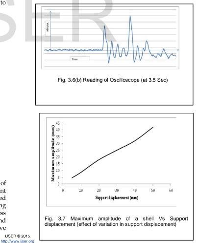
It is observed in fig. 3.14 that as the support displacement increases the amplitude of vibration increases. For support displacement of 5 mm the amplitude is 4.5mm while for value of support displacement 37 mm the amplitude is 42 mm and got the reading of 8 volts in the oscilloscope by our experiments. The stable time remains same for all values of support displacement.
